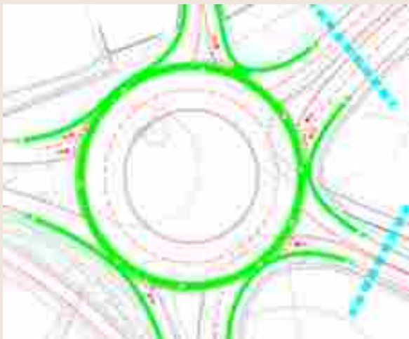
Figure 1a: Example of adjacent cycle lanes on local roundabout, proposed plan for Buqana roundabout.
