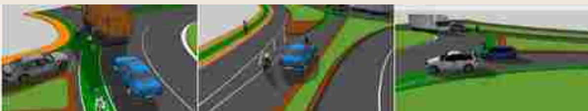
Figure 3a (left), 3b (middle) and 3c (right): Potential conflicts on roundabout with adjacent cycle lanes (drawn by author, Matthew Farrugia, based on Buqana roundabout plans).
